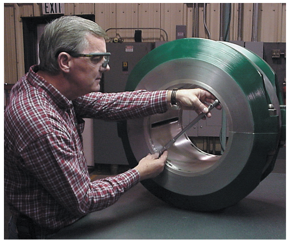
Centrifugally cast steam turbine bearing.
