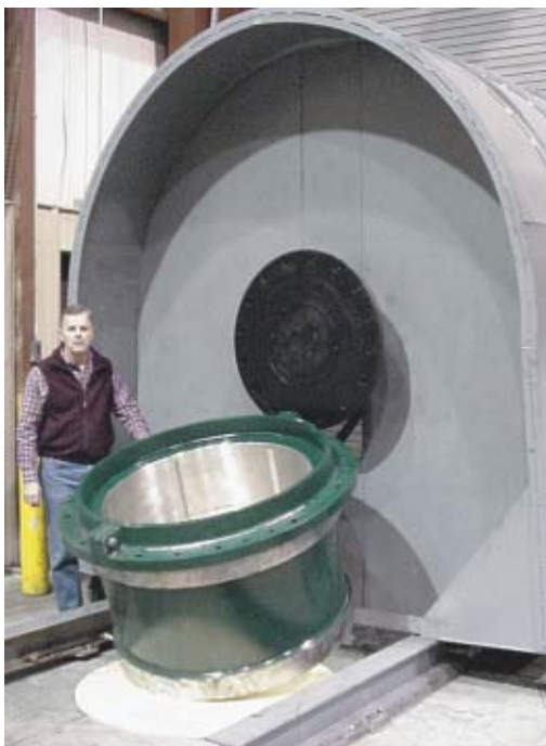
Spin Fixture to handle 120" O.D. up to 10,000 lbs.
