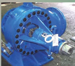
Impco 600 High Shear Mixer Use: Bleach Plant (SS, Hast C, or Titanium)
